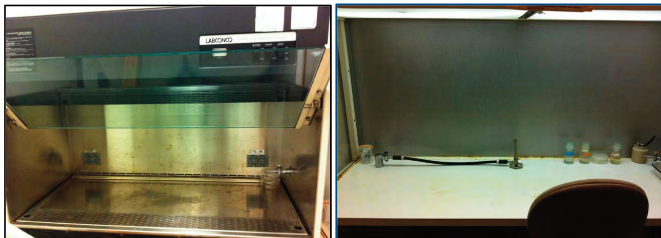
Figure 2-11. Two types of clean hoods. Left, a biological safety cabinet, suitable for working with cultures or hazardous materials. Right, a laminar flow cabinet, suitable for working with cultures and non-hazardous materials.
