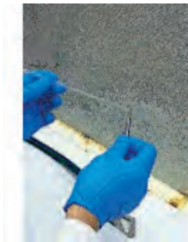
2) Pull ends apart to stretch glass.
